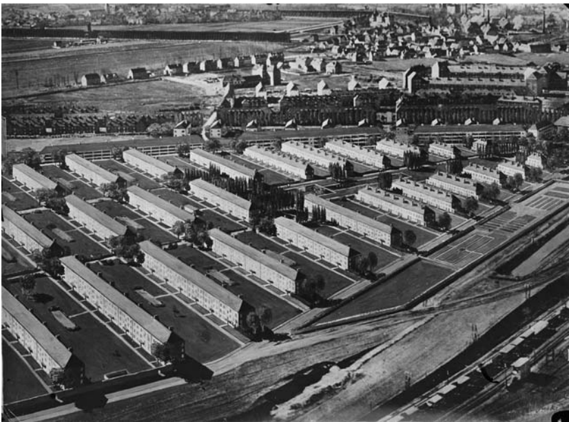
Fig. 6. Alexander Klein, aerial view of the rigid Zeilenbau of workers' settlement Bad Dürrenberg near Leipzig based on an earlier master plan by Walter Gropius, 1928–1930. (Photo: Bundesarchiv, Bild 102-09733.)
